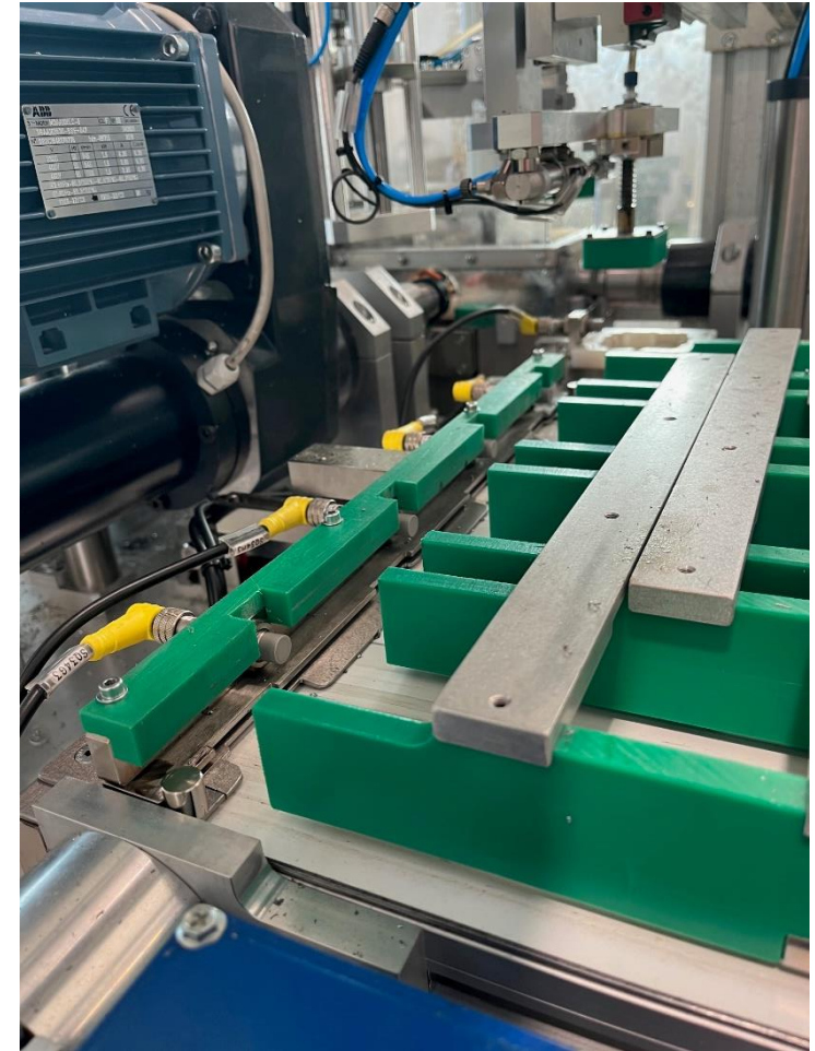
Suction cup call for loading pieces into limit switch production line
