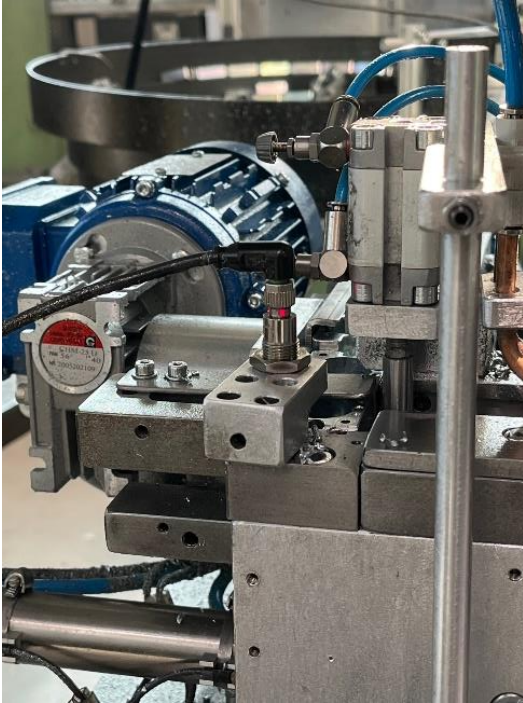
Detection of pieces on a track of an automatic line for the production of pushbuttons
