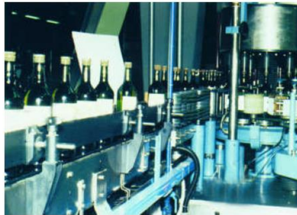
Detection of the presence of metal caps on the bottles
